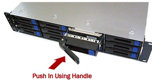
**IMPORTANT:** To maintain proper airflow and cooling, a drive assembly or a blank carrier must be installed in every bay. No empty bays are allowed.
